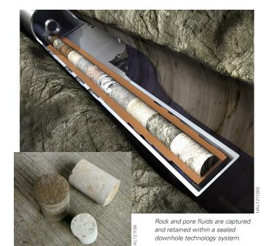
The Xaminer® Coring tool provides core samples that are 1.5 in. in diameter and 2.4 in. in length—more than three times the volume of other tools.
