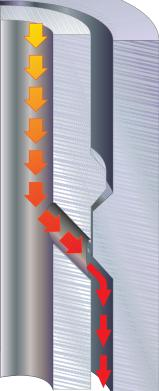
The HSB system consists of a heavy-duty outer assembly and a seated inner assembly. Outer tubes are 30 ft long for standard stability, 15 ft for extra stability. HSB is fully compatible with all types of Halliburton inner tubes and core heads.
