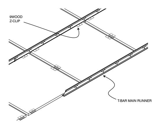
The **4100 Tegular Tile** wood ceiling offers a tiled appearance. The 4100 Tegular Tile hangs from and is accented by 9/16" standard black T-Grid. Reveals between panels are created by the width of the T-Bar flange (i.e., 9/16").
