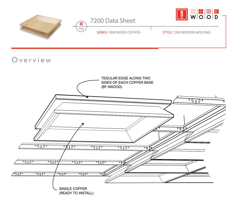
The 7200 Modern Molding Coffer style wood ceiling offers a coffer design typical of modern European woodwork. The coffer frame remains angular. The coffer lays into 15/16" standard T-Bar grid below the grid. Multiple veneer pattern options are available for the coffer interior panel.
