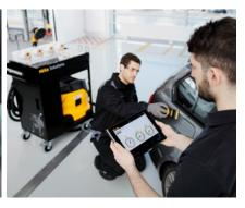
By using the **myMirka**<sup>®</sup> app you can monitor the vibration level when sanding with Mirka<sup>®</sup> DEOS.
