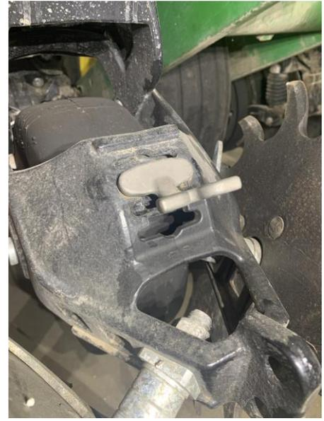
Figure 4. Reveal™ Depth Adjustment in Notch 1
