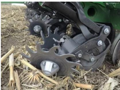
Figure 4. SmartFirmer Sensing Residue
