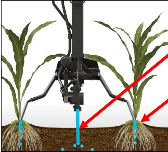
Center of Row Knife and Nozzle High Pressure Knife and Nozzle Injection
