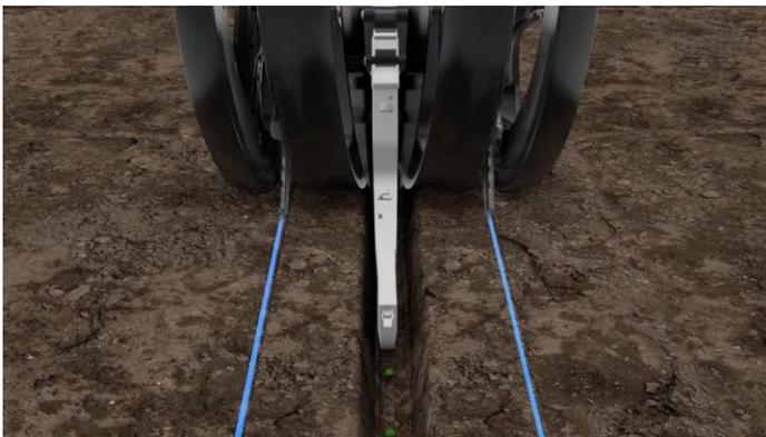
Figure 1. Conceal® Single or Dual Placement 3" from Seed Trench, 1.5" in Depth
