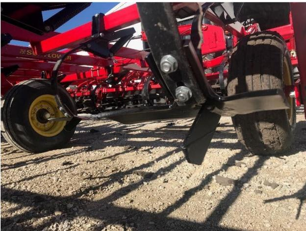
Figure 4. Finish™ Line Sweeps on 9" Spacing
