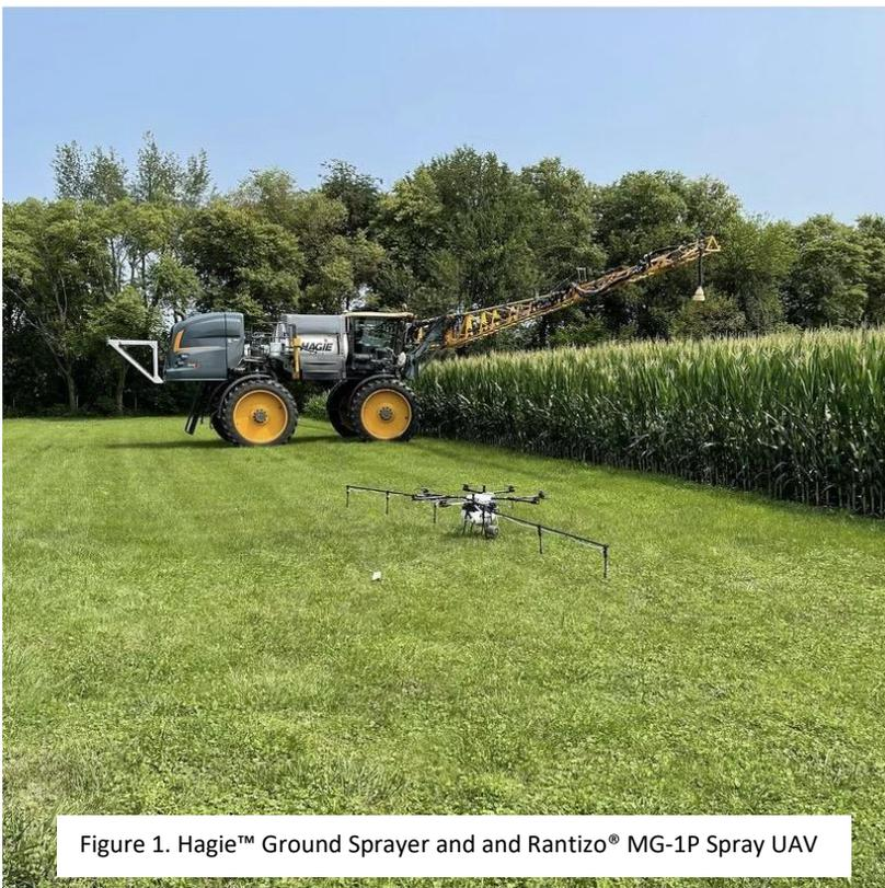
Figure 1. Hagie™ Ground Sprayer and Rantizo® MG-1P Spray UAV
