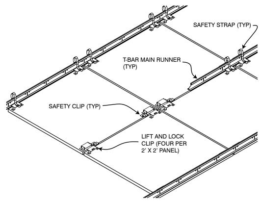
Designed with seismic zones in mind, the 4300 Lift & Lock<sup>™</sup> Tile wood ceiling offers a floating tiled appearance with a concealed suspension grid. The 4300 Lift & Lock<sup>™</sup> Tile is suspended from concealed 15/16" or 1-1/2" standard black T-Bar. Reveals between panels are 3/8" wide.
