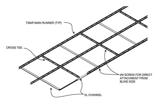
Designed with large wood panels in mind, the 4500 XL Channel Channel Tile wood ceiling offers a floating tiled appearance. The 4500 style installs progressively using perimeter extrusion clips (XL Channel). The reveal between panels are 3/8" wide.
