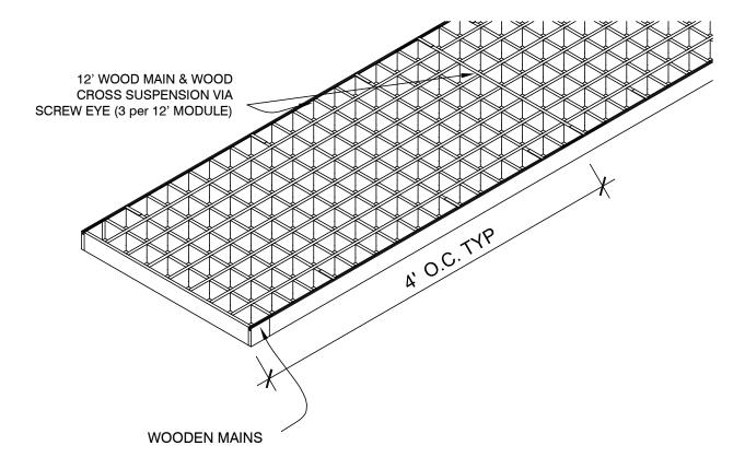
Designed with thin blades in mind, the 9Wood Monolithic Cube Wood Grid style wood ceiling offers a classic cell wood ceiling in a monolithic, continuous ceiling field. The 6600 Monolithic Cube Wood Grid style is suspended from matching wood suspension members. When the cube infill panel is installed, all members are flush A.F.F., creating a monolithic appearance. Without the size limitation of commercial T-Bar grid, thin solid wood blades can be used.
