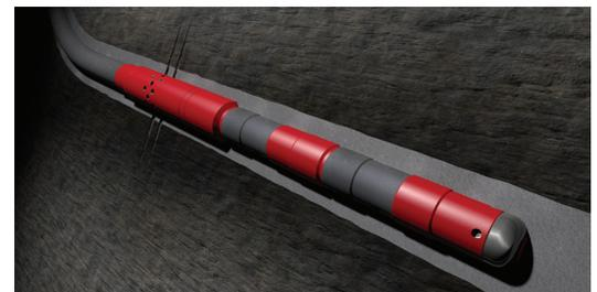
intervention trip by coiled tubing to perform toe preparation operations and create access to the formation by perforating with TCP guns or a hydra-jetting process so that multistage stimulation operations can be conducted.
