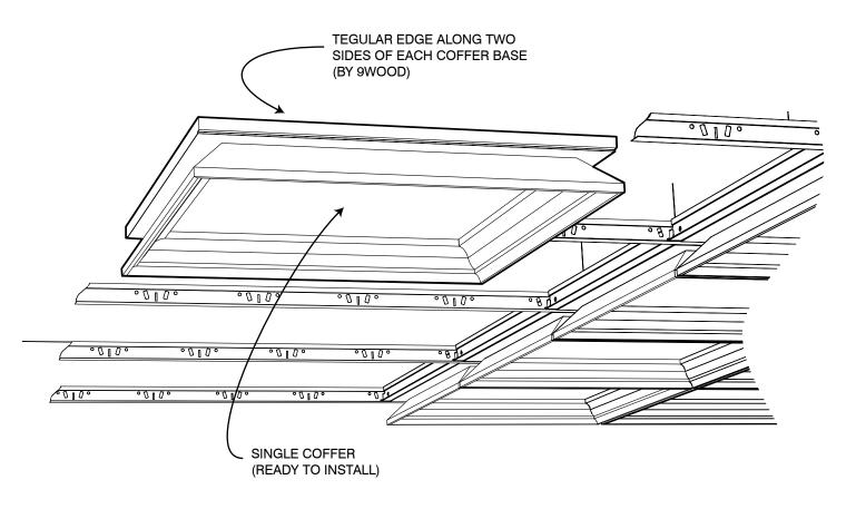
The **7100 Crown Molding Coffer** style wood ceiling offers a classic coffer profile typical of traditional woodworking. The coffer lays into 15/16" standard T-Bar grid below the grid. Multiple veneer pattern options are available for the coffer interior.
